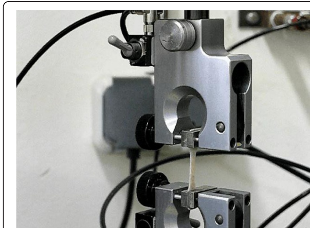
Figure 2 Sample clamped in the tensile testing machine.
